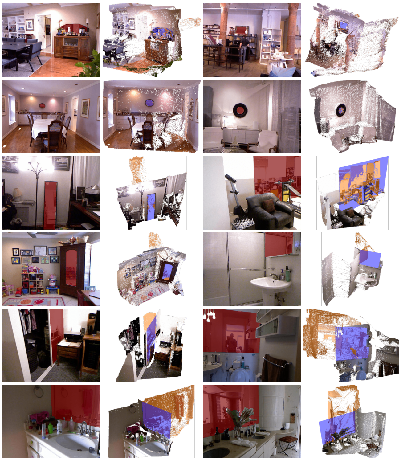
Figure 10: Example 3D mirror plane annotations in our Mirror3D dataset. Source RGBD data from the NYUv2 [32] dataset. In each image pair, the mirror mask is shown as a transparent red on the RGB image, the mirror plane is in light blue on the point cloud, and erroneous depth points that are incorrectly behind the mirror plane in the raw depth are shaded in orange.
