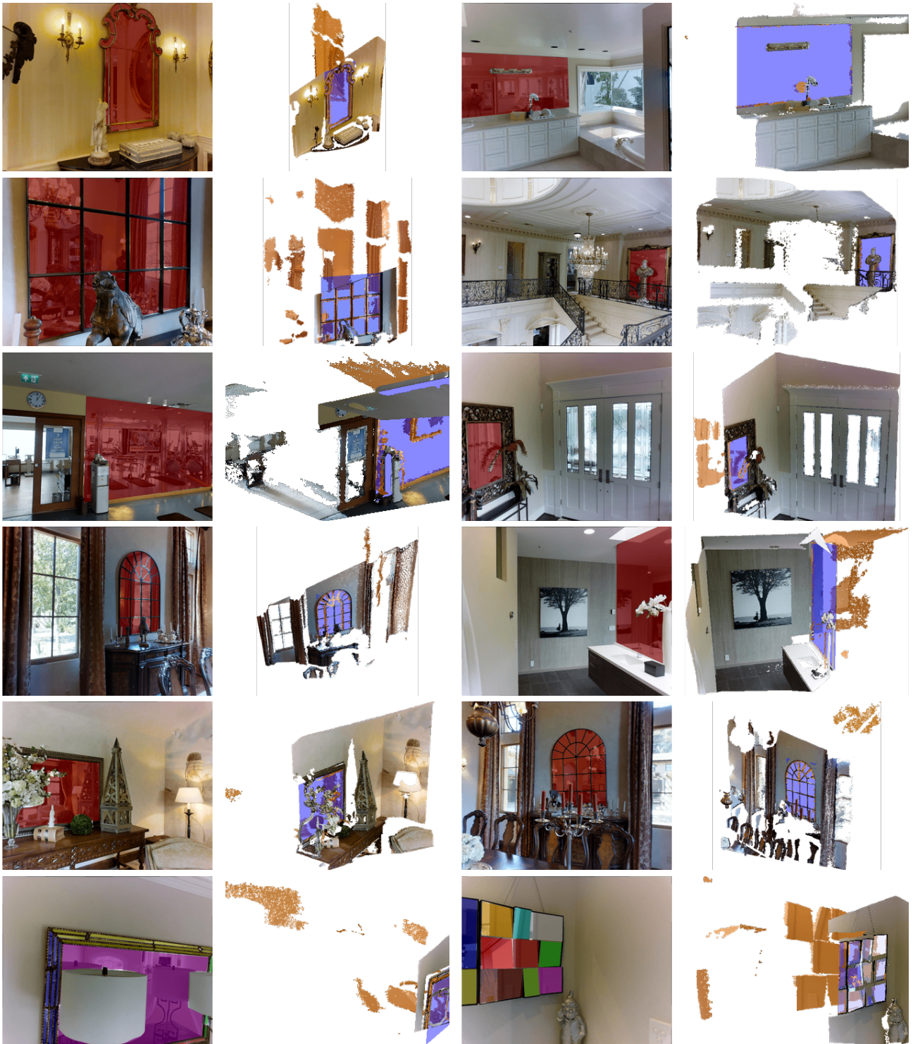
Figure 11: Example 3D mirror plane annotations in our Mirror3D dataset. Source RGBD data from the Matterport3D [6] dataset. In each image pair, the mirror mask is shown as a transparent polygon (with different color signifying each mirror instance) on the RGB image, the mirror plane is in light blue on the point cloud, and erroneous depth points that are incorrectly behind the mirror plane in the raw depth are shaded in orange.
